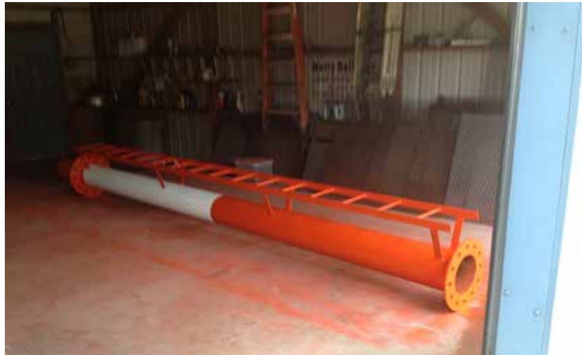
Bolt-together tower section with heavy flanges. NOTE: OSHA CLIMBING LADDER (NO DANGEROUS CLIMBING SPIKES LIKE THOSE FOUND ON OTHER POLE-TYPE TOWERS).
