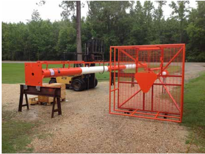
Towers have heavy base plate with gussets. NOTE: triangular beacon mounting platform.
