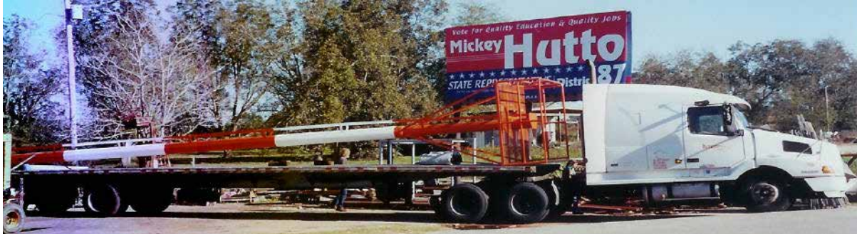
Standard FAA 51' beacon tower being shipped fully assembled on flatbed trailer. Towers are shipped FOB Hartford, AL USA 36344.
