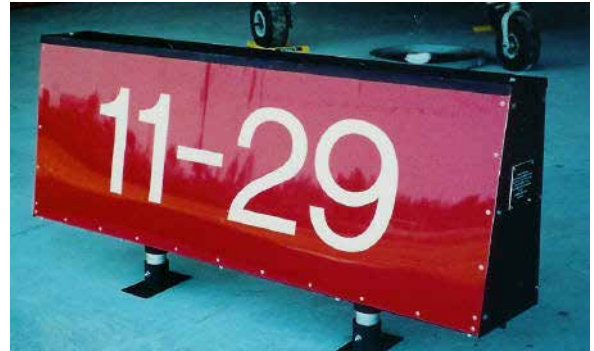
Mandatory "hold short", internally lighted sign.
