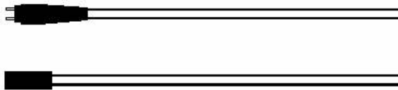
FAA L-823 cable plugs and female receptacles.
