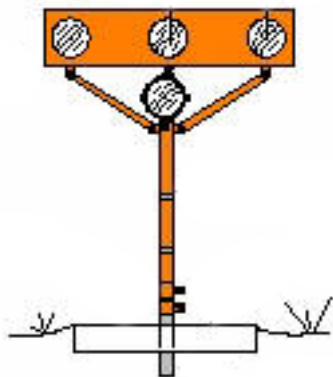
3 light approach light tower with attached sequence flashing light. (ICAO European-style)
